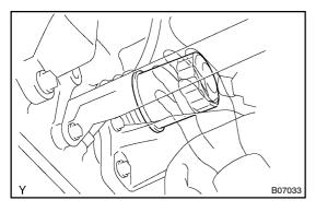
(e) Tighten the oil filter by hand until the rubber gasket contacts the seat of the filter mounting.
