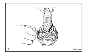
(c) Using a screwdriver, remove the 4th gear bearing inner race.
