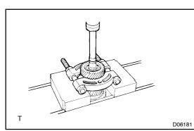
(b) Using SST and press, remove the counter gear. SST 09950-00020, 09950-60010 (09951-00230), 09950-70010 (09951-07010)
