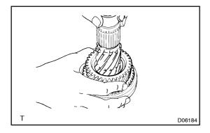
(d) Remove the counter shaft 4th speed gear and synchronizer ring No. 1.
