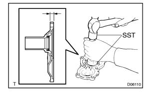
(b) Using SST and a press, install the new oil seal. SST 09950-60010 (09951-00420), 09950-70010 (09951-07100)
