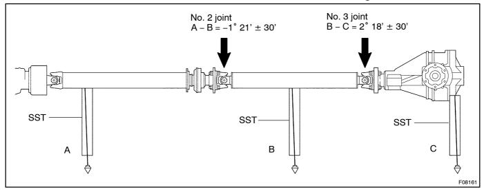
If the measured angle is not within the specification, adjust it with the center support bearing adjusting washer and differential adjusting shim.
