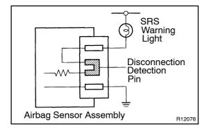
(3) Electrical connection check mechanism:
