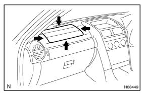
There should be no interference between the instrument panel and front passenger airbag assembly.
