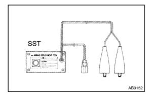
When deploying the airbag, always use the specified SST (SRS Airbag Deployment Tool). Perform the operation in a place away from electrical noise.
