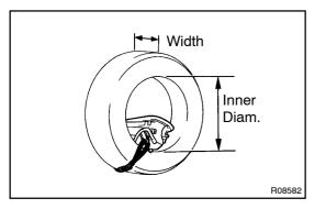
(2) Position the front passenger airbag assembly inside the tire with the airbag deployment side facing inside. Tie the front passenger airbag assembly to the tire, as shown in the illustration.
