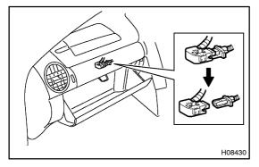
(b) Disconnect the front passenger airbag assembly connector.
