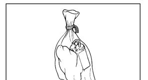
(g) Dispose of the front passenger airbag assembly.
