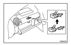
4. CONNECT FRONT PASSENGER AIRBAG ASSEMBLY CONNECTOR
