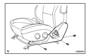
7. Manual adjuster type: REMOVE FRONT SEAT CUSHION SHIELD Remove the 3 screws and front seat cushion shield.
