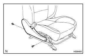
9. Manual adjuster type: REMOVE FRONT SEAT CUSHION INNER SHIELD Remove the 2 screws and front seat cushion inner shield.
