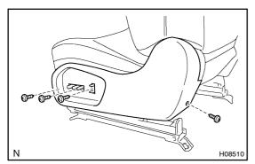
6. Power adjuster type: REMOVE FRONT SEAT CUSHION SHIELD
