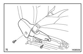
8. Power adjuster type: REMOVE FRONT SEAT CUSHION INNER SHIELD Remove the 2 screws and front seat cushion inner shield.
