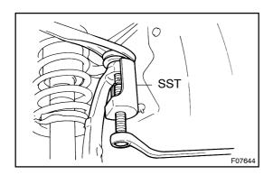
(b) Using SST, remove the steering knuckle from the upper suspension arm.
