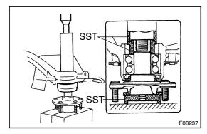
Using SST and a press, install the axle hub to the steering (b) knuckle.
