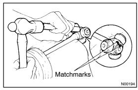
(b) Place matchmarks on the drive shaft and tripod.
