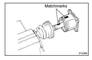
(b) Place matchmarks on the inboard joint tulip and drive shaft.
