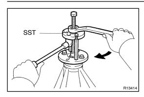
(c) Using SST, install the companion flange. SST 09950-30011 (09951-03010, 09953-03010,
