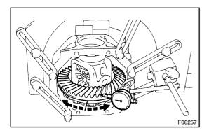
(f) Using a dial indicator, while holding the companion flange adjust the ring gear backlash until it is within the specified value.
