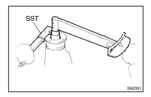
(c) Using SST to hold the flange, tighten the nut. SST 09330-00021
