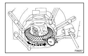
(j) Using a dial indicator, while holding the companion flange measure the ring gear backlash.
