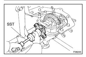
(c) Using SST and the 2 nuts, install the 2 side gear shafts to the differential carrier.
