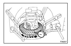
(c) Using a dial indicator, while holding the companion flange, measure the ring gear backlash.
