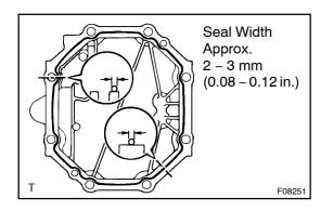
(e) Apply FIPG to the carrier cover, as shown in the illustration.
