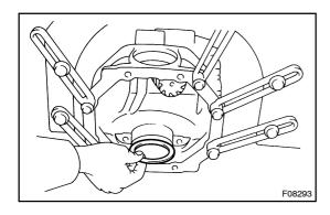
(g) Install the plate washer into the ring gear back side of the carrier.
