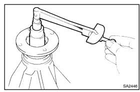
(e) Using a torque wrench, measure the drive pinion preload using the backlash between the drive pinion and ring gear.
