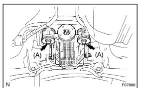
(b) Support the rear differential carrier assembly with a jack and temporally install the lower mount stoppers and 2 new bolt (A).
