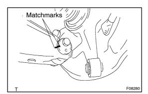
(b) Connect the No. 2 lower suspension arm to the axle carrier with the cam bolt, cam plate and nut.
