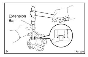
(b) Using a plastic hammer and extension bar, lightly tap in a new union seat.
