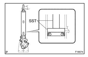
(c) After the oil seal has passed through the ports, push in the oil seal by hand until it becomes level, using SST.
