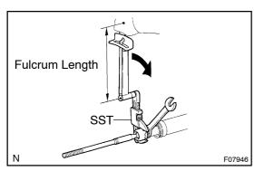
(b) Using a spanner, hold the steering rack steadily and using SST, torque the rack end.
