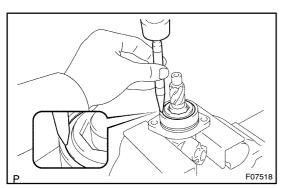
(c) Using a punch, stake the bearing guide nut.
