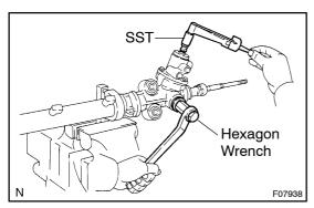
(f) Using SST, a torque wrench and hexagon wrench (24 mm), tighten the rack guide spring cap until the preload is within the specification.
