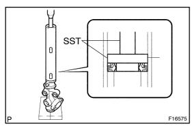
(d) After the oil seal has become level, using SST and press, install the oil seal.
