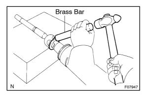
(c) Using a brass bar and a hammer, stake the washer.
