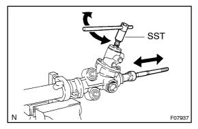
(d) Using SST, turn the control valve shaft right and left 1 or 2 times.
