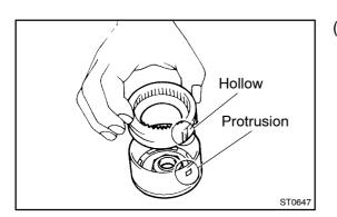
(c) Align the hollow of the internal gear with the protrusion inside the shock absorber, and remove the internal gear.
