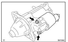
(b) Remove the 2 nuts holding the magnetic switch to the starter housing.
