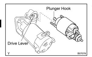
(c) Pull the magnetic switch, and disconnect the plunger hook from the drive lever and remove the magnetic switch.
