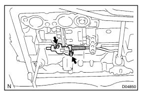
**21. REMOVE PARKING LOCK PAWL BRACKET** Remove the 2 bolts and parking lock pawl bracket.
