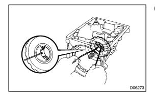
(b) Insert the 2 wires into the planetary gear nd remove it.
