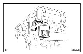
2. REMOVE SOLENOID WIRE RETAINING BOLT NOTICE: Remove the bolt only and do not remove the solenoid wire.
