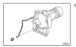
(c) Remove the gasket and oil apply pipe from the extension housing.
