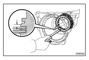
**32.** CHECK PACK CLEARANCE OF NO. 3 BRAKE Using calipers, measure the clearance between the disc and transmission case, as shown.
