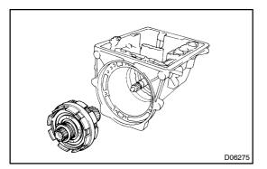
(b) Remove the center support form the transmission case.
