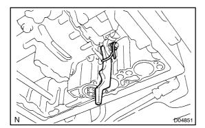
22. REMOVE SPRING, PARKING LOCK PAWL PIN AND PARKING LOCK PAWL
