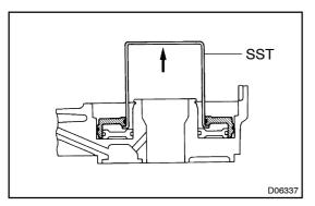
(f) Insert SST behind the reaction sleeve and gradually lift it out of the transmission case.
