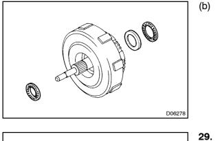
(b) Remove the 2 bearings and race.
