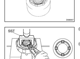
(b) Place SST on the spring seat, and compress the return spring with a shop press.
