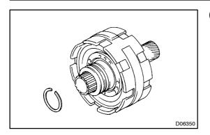
(b) Using a snap ring expander, install the snap ring.
