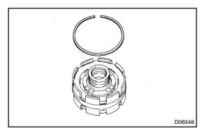
(b) Using a screwdriver, install the snap ring. Be sure the end gap of the snap ring is not aligned with the cutout portion of the center support.
