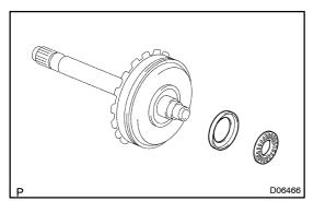
(b) Remove the bearing and race.
