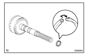
**8. REMOVE OIL SEAL RING FROM OUTPUT SHAFT** Remove the oil seal ring.
