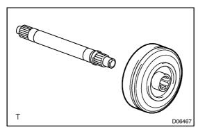
(b) Remove the planetary ring gear.
