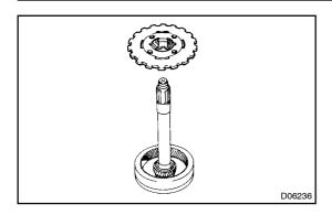
4. REMOVE REAR PLANETARY CARRIER FROM PLAN-ETARY RING GEAR
