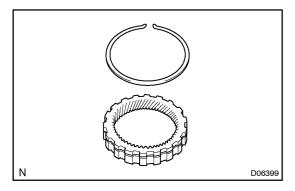
(b) Using a screwdriver, remove the snap ring from the ring gear.
