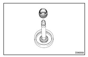
5. REMOVE PLANETARY SUN GEAR FROM PLAN-ETARY RING GEAR
