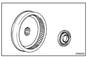
(c) Remove the assembled bearing from the ring gear.
