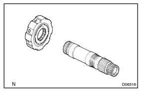
3. REMOVE NO. 1 ONE-WAY CLUTCH FROM PLAN-ETARY SUN GEAR
