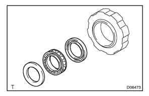
(c) Remove the one–way clutch and 2 retainers from the outer race.
