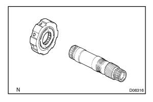
3. INSTALL NO. 1 ONE-WAY CLUTCH TO PLANETARY SUN GEAR
