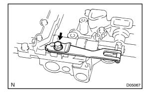
1. REMOVE DETENT SPRING AND SPRING PLATE Remove the bolt, detent spring and spring plate.
