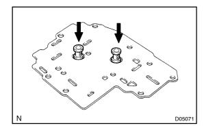
(d) Remove the 2 strainers from the plate sub assembly.
