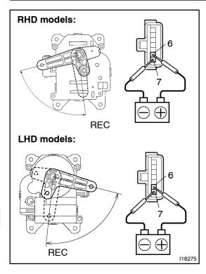
(b) Connect the positive (+) lead from the battery to terminal 6 and negative (-) lead to terminal 7, then check that the arm turns to "RECIRC" side smoothly.
