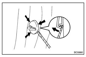
(b) Using a screwdriver, remove the striker cover.
