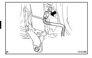
(1) Disconnect the pretensioner connector as shown in the illustration.
