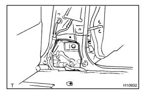
Check for deformation of the center pillar.
