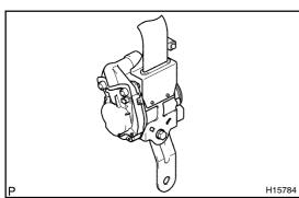
Check for cuts and miute cracks in wire harness or marked discoloration on the front seat outer belt.
