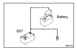
Connect the SST to the battery.
