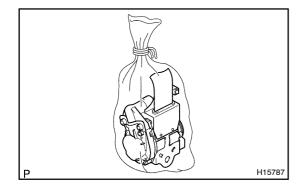
(f) Dispose of front seat outer belt (with seat belt pretensioner).
