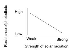
A photo diode in the solar sensor detects solar radiation and sends signals to the A/C control assembly.
