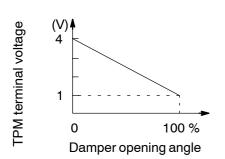
This sensor detects the position of the air mix damper and sends the appropriate signals to the A/C control assembly. The position sensor is built into the air outlet damper control servomotor assembly.
