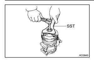
(3) Using SST and a torque wrench, install the shaft bolt.
