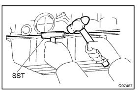
(b) Install the blade of SST between the transmission case and oil pan, cut off applied sealer, and remove the oil pan. SST 09032–00100
