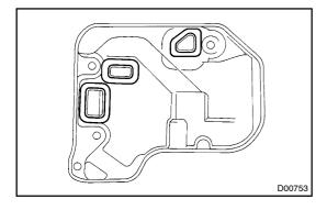
(b) Remove the 3 gaskets from the oil strainer.
