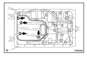
(b) Install the oil strainer with the 4 bolts.
