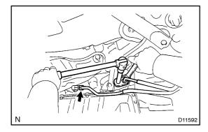
(b) Loosen the 2 union nuts from the transmission.
