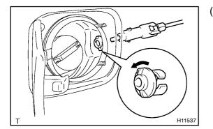
(b) Rotate the retainer left to disengage the lock, then pull it out.
