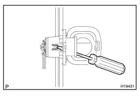
(b) Using a screwdriver, disengage the claw on the accessory socket cover from the body and remove the accessory socket and cover as a unit.
