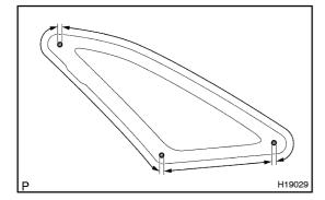
(e) Cut the adhesive by pulling the piano wire around it. HINT:
