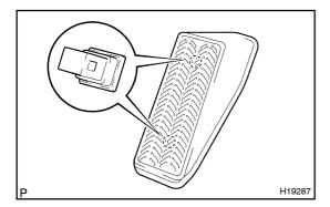
(b) Using a screwdriver, remove the foot rest.
