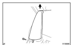
(d) Remove the bolt and the side seat back assembly as shown in the illustration.
