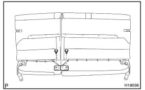
9. INSTALL REAR SEATBACK CENTER HINGE Install the rear seat center hinge with the 2 bolts. Torque: 21 N·m (214 kgf·cm, 15 ft·lbf)
