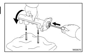
(b) Push in the piston with a screwdriver, and remove the 2 straight pins by turning over the cylinder body.
