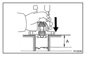
(d) Place a rag and 2 wooden blocks on the work table and lightly tap the cylinder flange against the block edges until the piston drops out of the cylinder.
