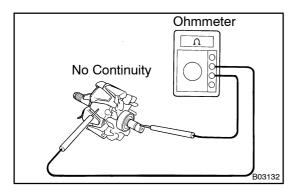
(b) Check the rotor ground.
