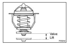
(c) Check the valve lift.
