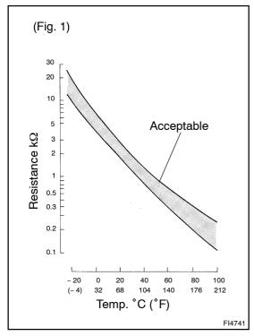
The intake air temperature sensor is built into the air cleaner and senses the intake air temperature.
