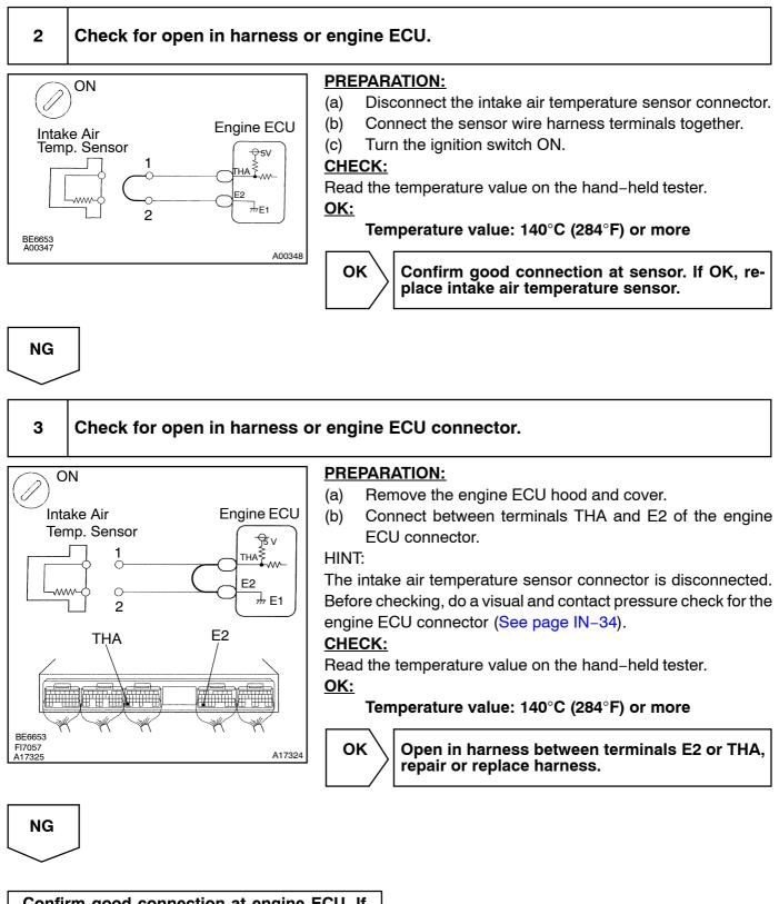
Confirm good connection at engine ECU. If OK, check and replace engine ECU (See page IN-34).
