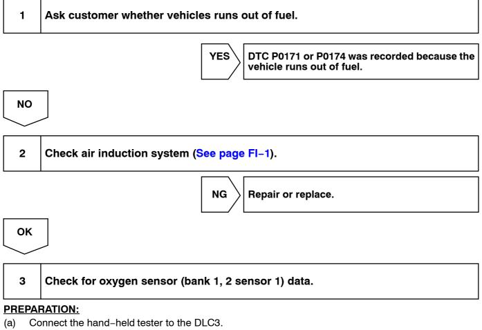
(b) Warm up the engine to normal operating temperature.
