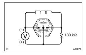
(a) Connect the 3 dry batteries of 1.5 V in series.
