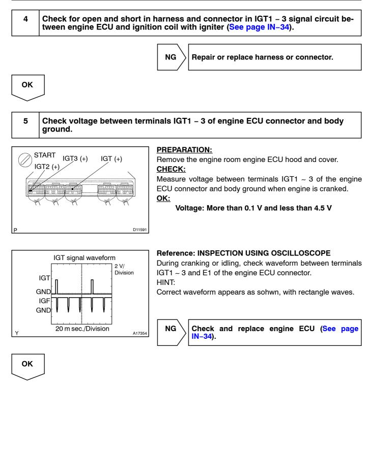
Disconnect connector and check voltage between terminals IGT1 – 3 of engine
