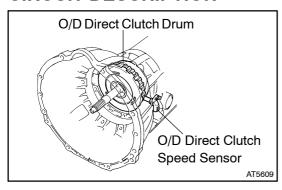
This sensor detects the rotation speed of the O/D input shaft from the rotation of the O/D direct clutch drum.
