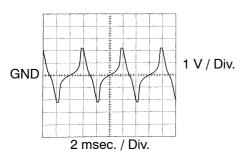
Refer to the chart for the wave form between terminals NC0<sup>+</sup> and NC0<sup>-</sup> during engine idling.
