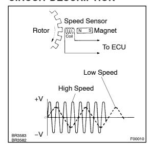
The speed sensor measures wheel speed and sends the corresponding signals to the ECU. These signals are used for control of both the ABS & TRC control system. Both the front and rear rotors have 48 serrations.
