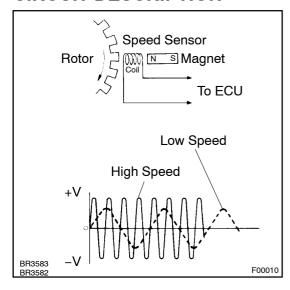
The speed sensor measures wheel speed and sends the corresponding signals to the ECU. These signals are used for control of both the ABS & TRC & VSC control system. Both the front and rear rotors have 48 serrations.
